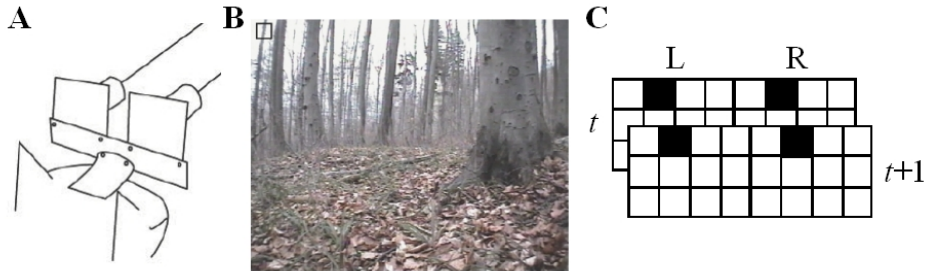
Figure 3: Description of stimuli. A Setup of the cameras on a cats head. B Example of a raw image recorded with one camera. Image is converted to greyscale before further processing. C Schematic representation of choice of patches for one stimulus configuration within optimisation. From left and right images of frame t and t + 1 one patch is chosen from a randomly drawn common position.
