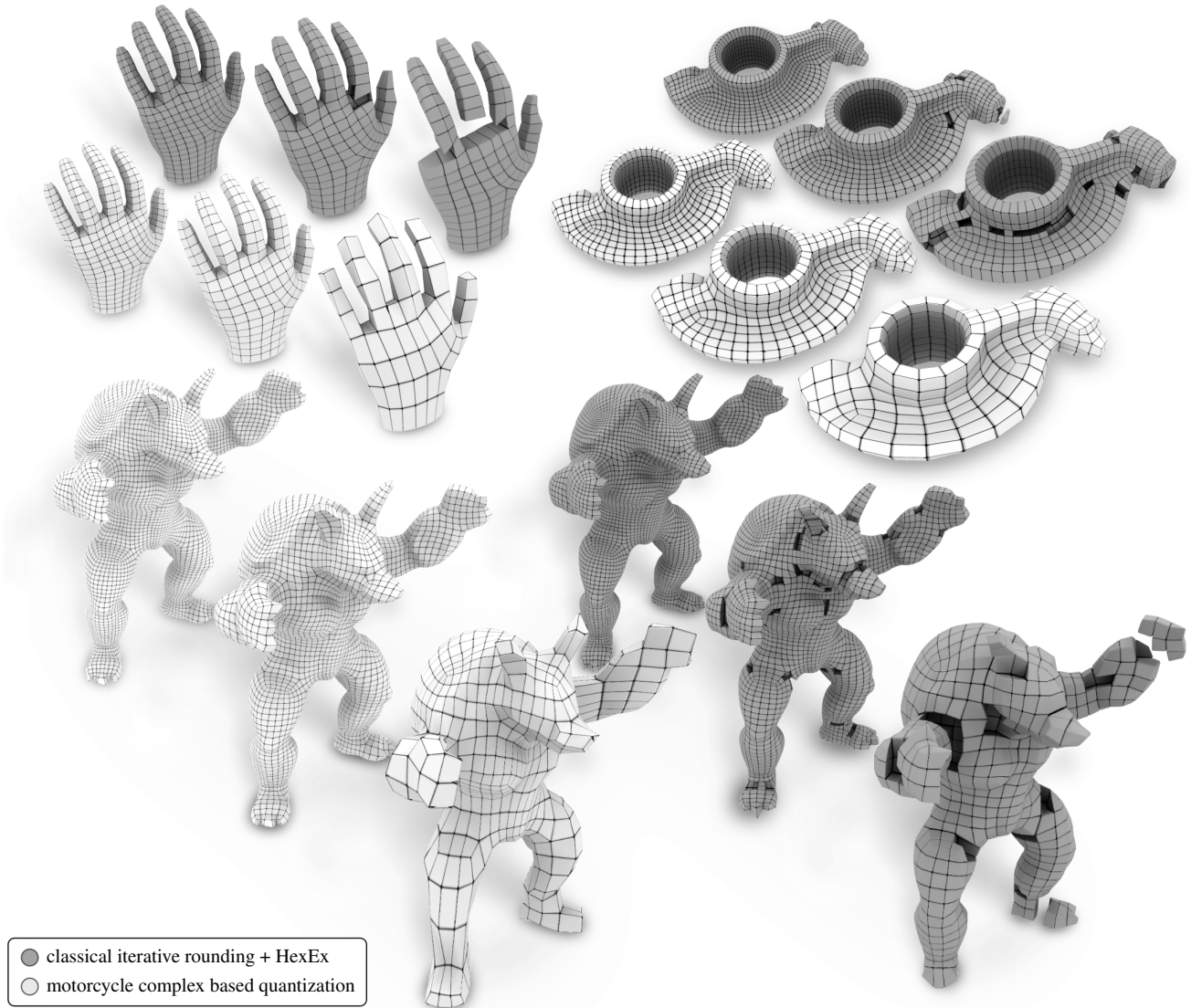
Figure 16: Hexahedral meshes of increasing coarseness obtained from seamlessly parametrized tetrahedral meshes by means of iterative rounding to an integer-grid map as described by [NRP11] (dark gray) and our method using the motorcycle complex (white). When increasing target coarseness, hexahedral meshes obtained by rounding become increasingly defective due to parametric degenerations and inversions. Even fault-tolerant mesh extraction [LBK16], as employed here, cannot recover from this, leaving gaps that cannot easily be patched.
